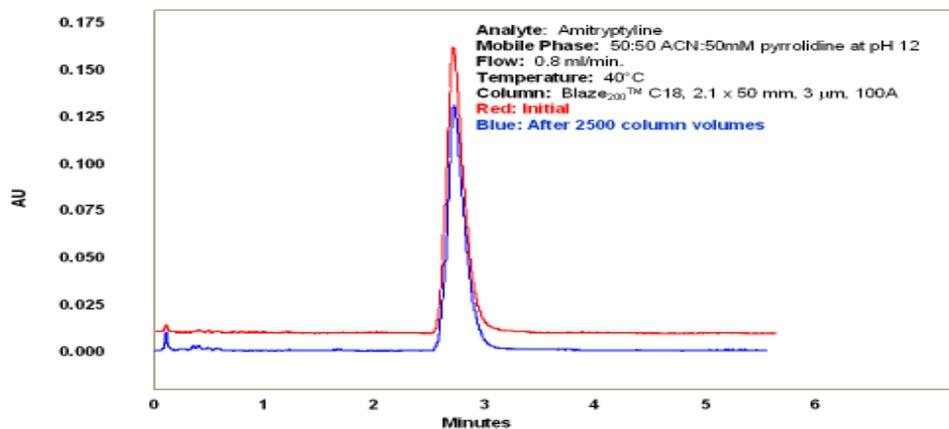
Figure 3. Chromatogram showing amitriptyline peak with new Blaze<sub>200</sub> column and after flushing with 2500 column volumes of pH 12 mobile phase..
