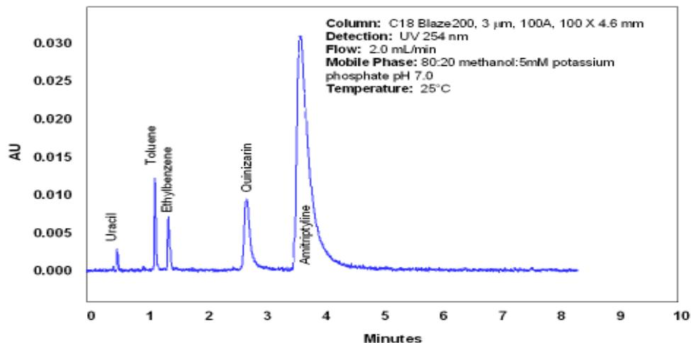
Figure 1. SRM 870 test conditions were followed, and indicate typical C18 silica column selectivity. Tailing and asymmetry for amitriptyline indicate some silanol interaction. Peak shape and elution of quinizarin indicate low activity toward metal chelating agents.
