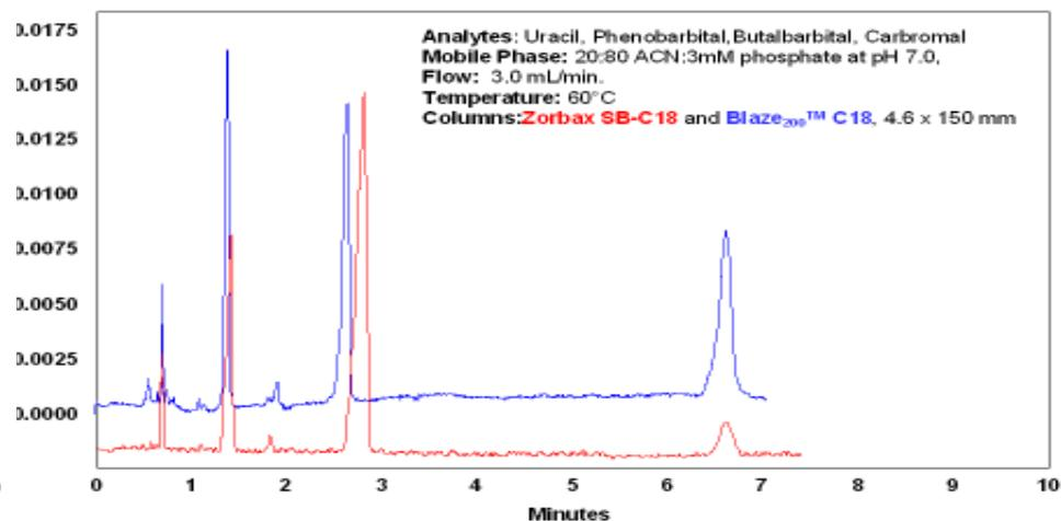
Figure 2. Selectivity comparison of the Blaze<sub>200</sub> C18 column and the Zorbax StableBond C18 for a mixture of barbiturates.
