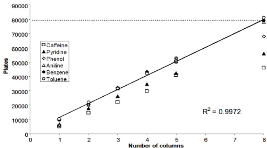
Figure 3. Plot showing the linear relationship between theoretical plates and column length.
