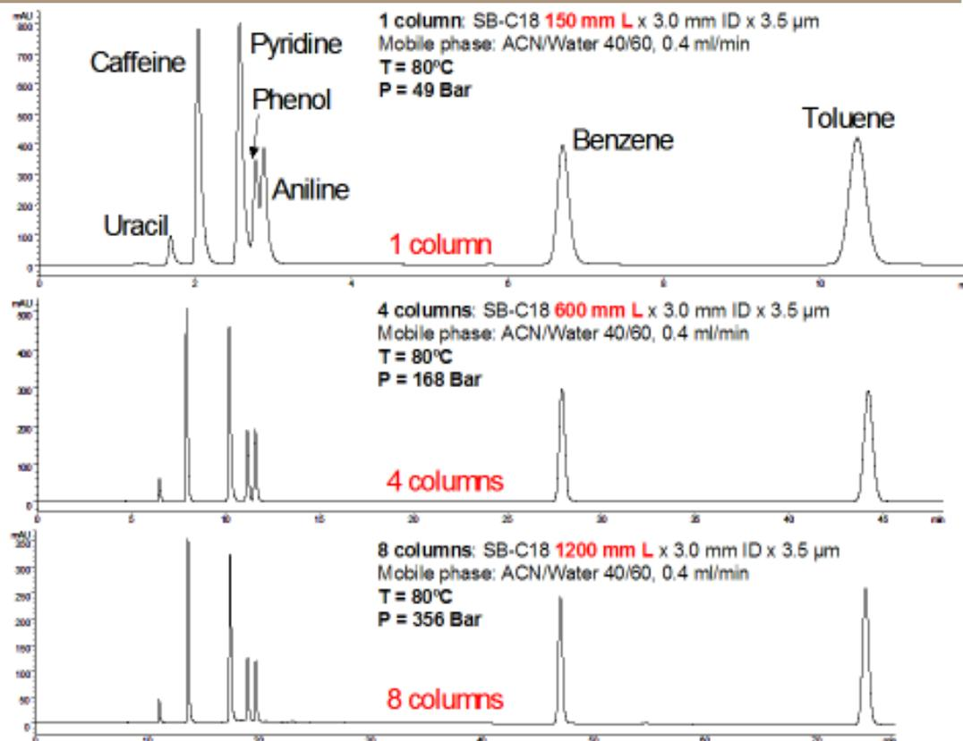
Figure 2. The separation of standard mix using one, four and eight columns. Resolution and efficiency are greatly increased by coupling columns together. Back pressure is still within normal limits, even with eight columns
