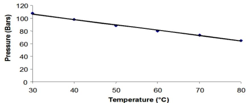
Reduction of pressure with temperature
