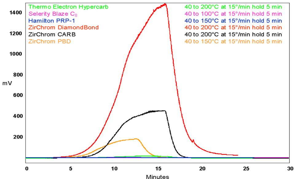
Figure 1. Blank temperature programs for the six columns studied. The Blaze™ C<sub>8</sub> and the PRP-1® showed essentially no column bleed. The Hypercarb® column showed a slight rise in the baseline. The three zirconia stationary phases had excessive column bleed.
