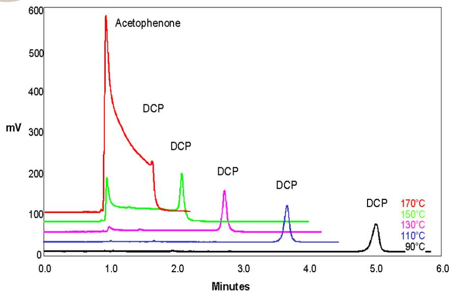
FIGURE 1: Decomposition of DCP at 1.0 mL/min
