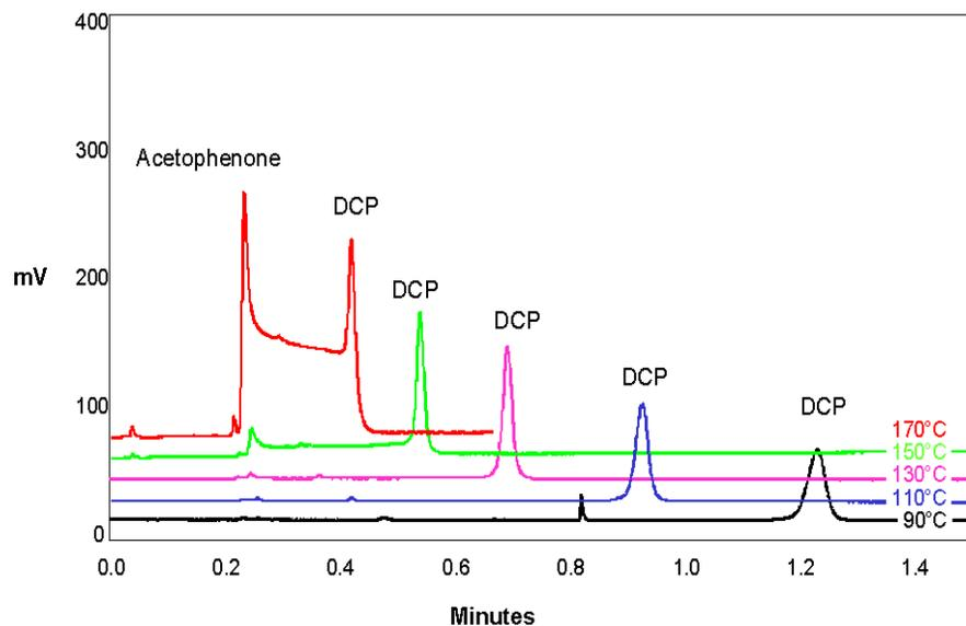
FIGURE 3: Decomposition of DCP at 4.0 mL/min
