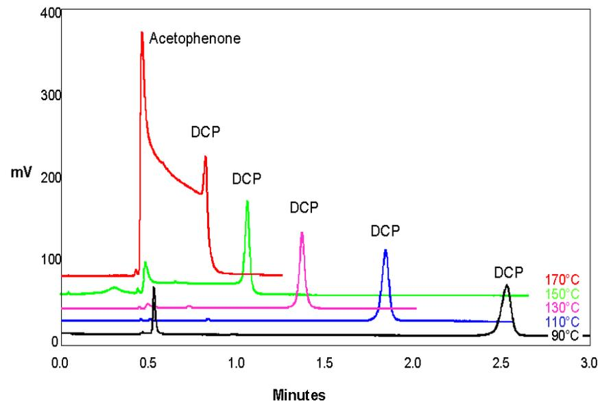
FIGURE 2: Decomposition of DCP at 2.0 mL/min
