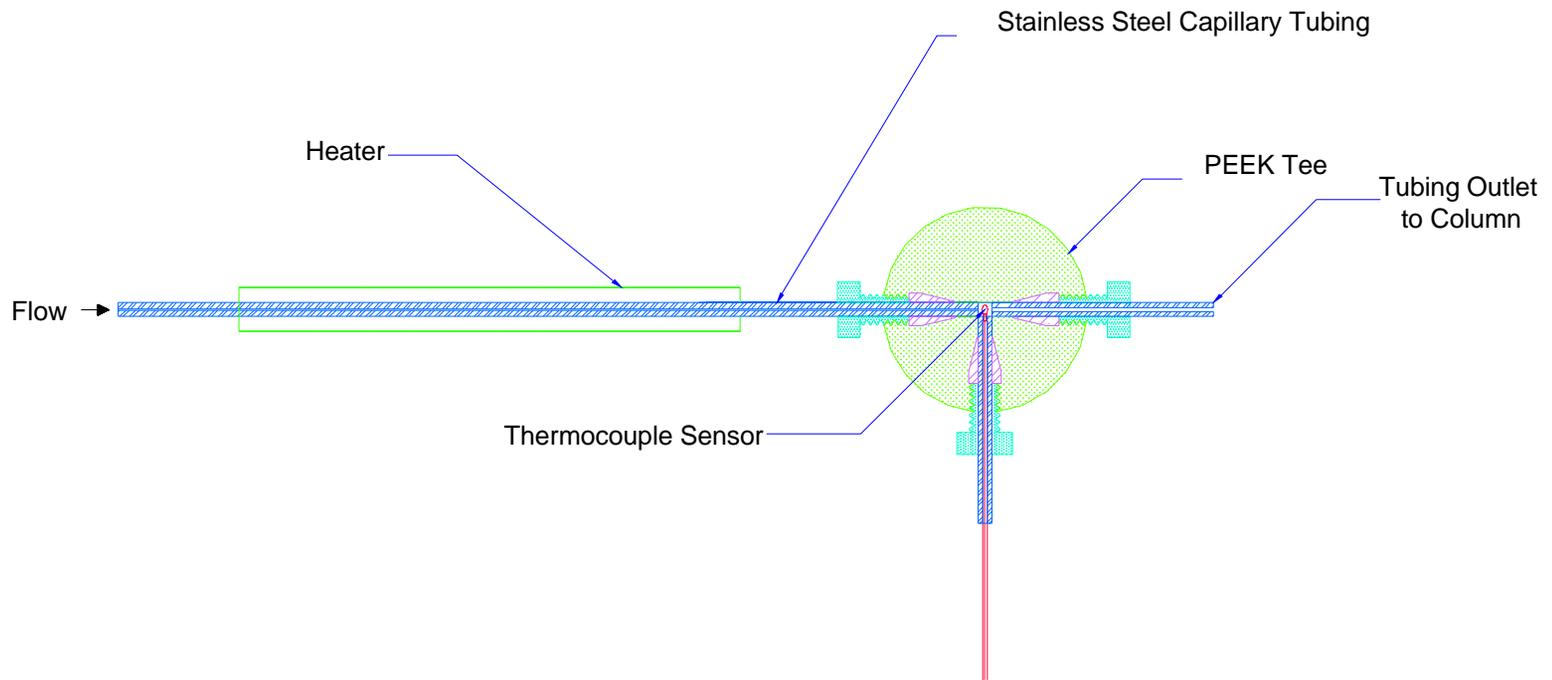
Invasive sensing with feedback control to a heater attached to the stainless steel tube leading to the column (Ref 3).
