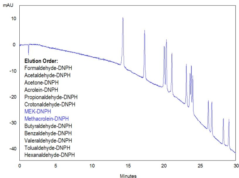
Figure 1: Solvent gradient analysis of aldehydes and ketones.
