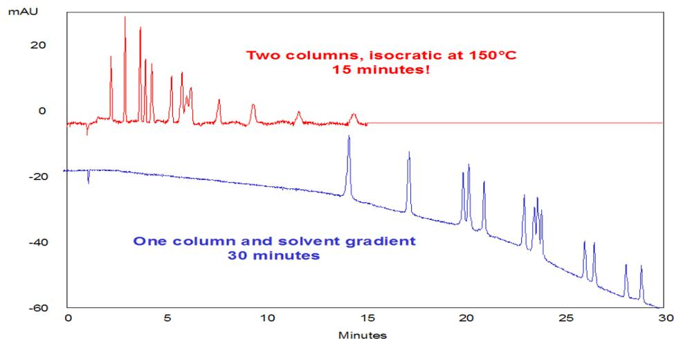
Figure 3: Overlay of the two analysis methods. Run time has been reduced to 15 minutes using the high temperature isocratic method.
