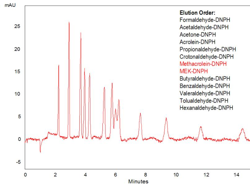
Figure 2: Isocratic high temperature method for aldehydes and ketones using two columns in series at 150°C.
