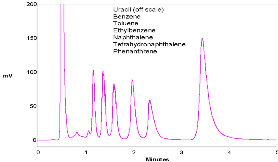
Chromatogram showing the separation of seven aromatic hydrocarbons using a temperature gradient from 50°C to 150°C at 20°C/min, holding at 150°C for two minutes.
