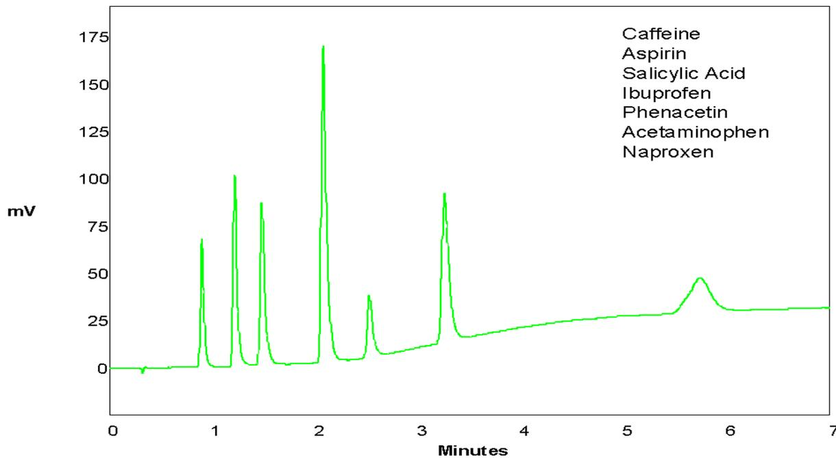
FIGURE 2: Separation of over-the-counter analgesics using a Hypercarb<sup>®</sup> column and a thermal gradient from 125°C to 200°C.
